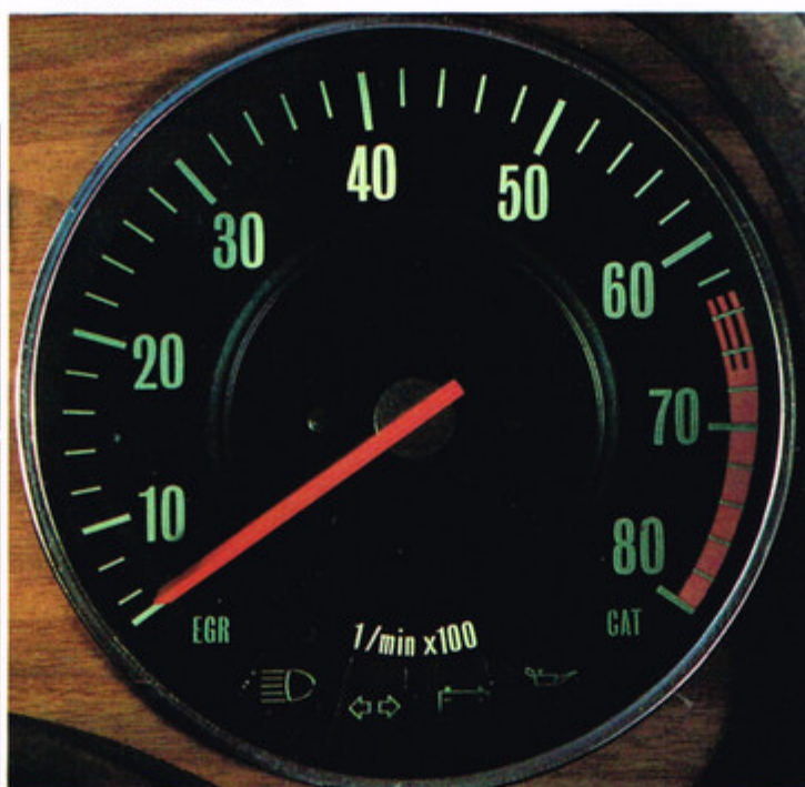
Large tachometer allows constant monitoring of engine speed.
