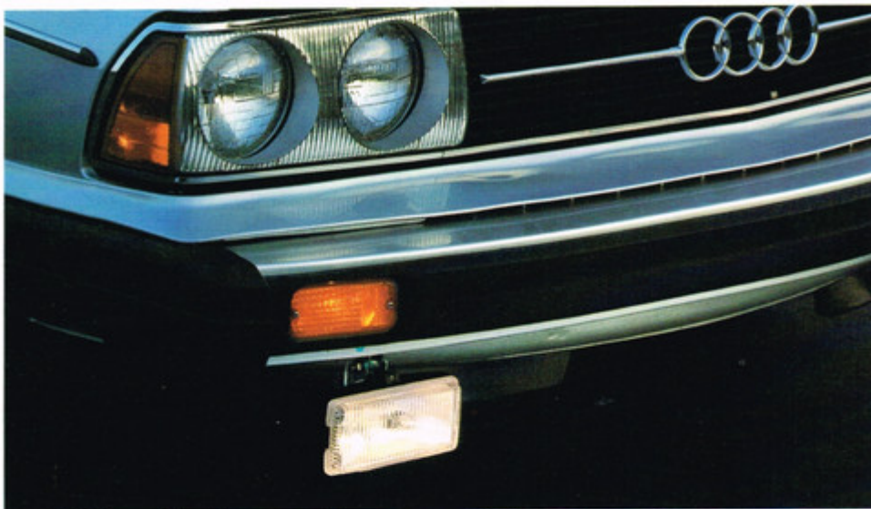
High intensity Halogen fog lamps, mounted close to the road for maximum effectiveness.
