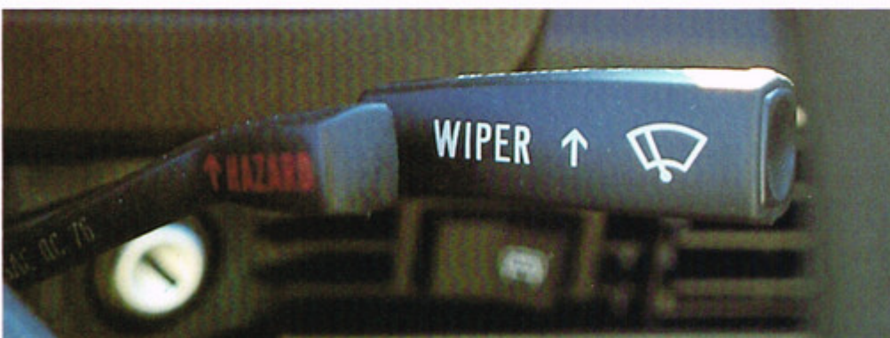
Stalk controls 2-speed wiper/washer and intermittent wiper cycle.
