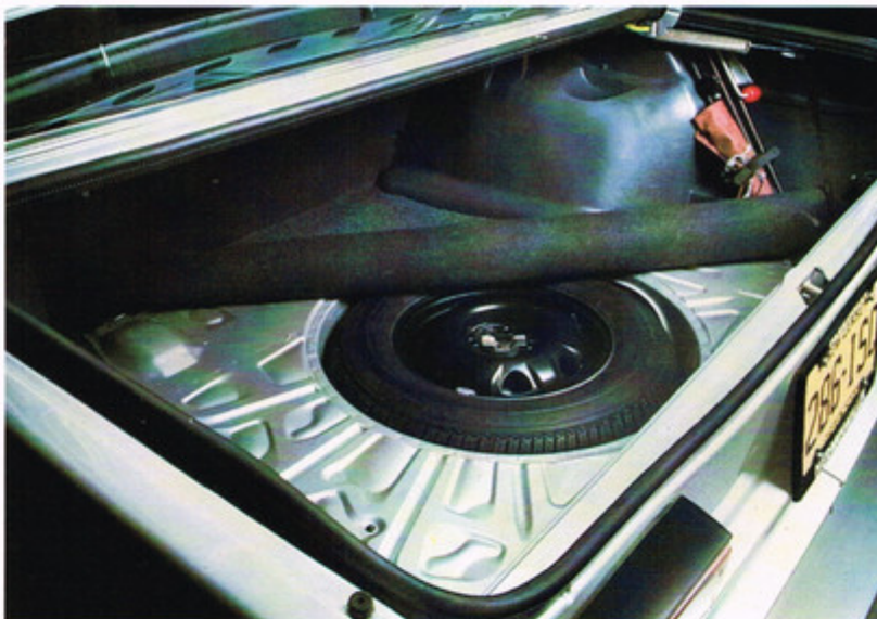
Spare tire stows away in a well beneath the trunk floor.
