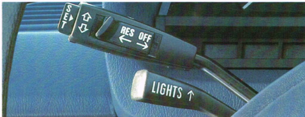
Larger, multi-function stalk includes cruise control, turn signal indicator, headlight dimmer, and passing light. Smaller lower stalk controls the headlights.
