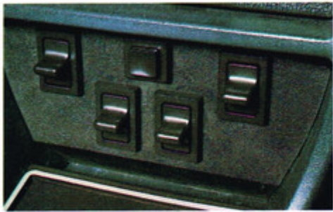
Center console with power window and rear window power lock control.
