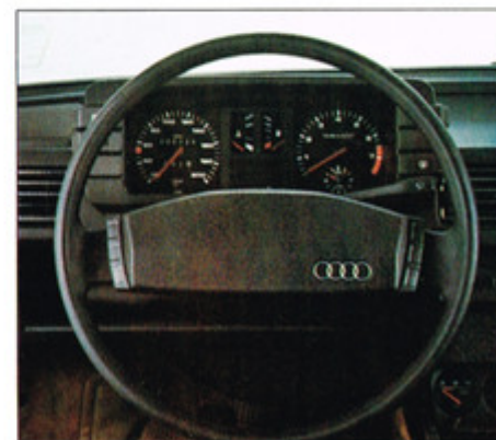
4000 instrumentation includes a tachometer, trip odometer, quartz clock, voltmeter and oil temperature gauge.
