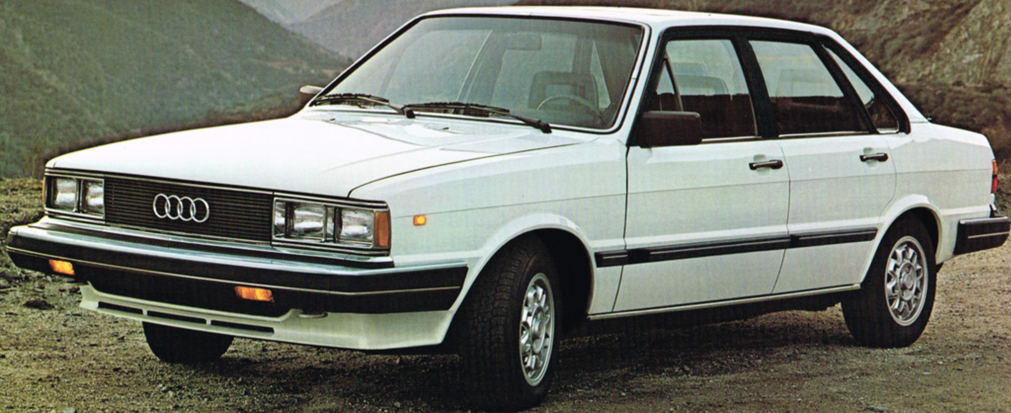
The Audi 4000 Turbo-Diesel sedan. Available in 4-door body style only—with either 5-speed manual or optional E-mode automatic transmission. Distinctive Audi light-alloy wheels, air-own, are standard with the 4000 Turbo-Diesel. With 5-speed, zero - 50 mph is a brisk 8.8 seconds. Top track speed, 98 mph.
